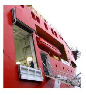
**ROV side-hangar doors** are designed to function in adverse weather and heavy seas whilst ensuring continuity of ship operations. Design options are available to cater for a variety of operator needs. Door selection takes into consideration ship design, method of ROV launch and sea-state. Controls may be integrated into the control system of the Launch-and-recovery systems (LARS) for simplified operation
