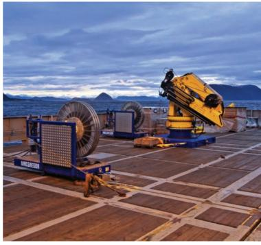
Deck-skid system with hydraulically driven tractor units, pallets and full deck rail arrangement enable safe, controlled shuttling of loads of up to 100 tonnes, across open deck, into multiple ship hangars and across moonpools even while underway.
